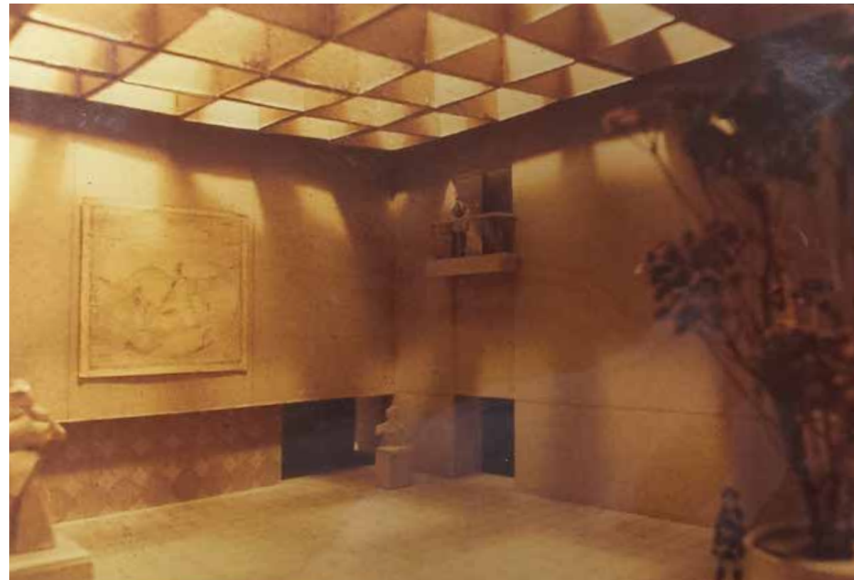
Above: Architectural models were built to study the effects of natural light in the building. This model shows the ceiling coffers in the model that were fully articulated and could be rotated on the ceiling grid upon which they rested. The model allowed architects to test different directions of light for the galleries. The final choice was a northern skylight orientation, which is shown in this picture. Top right: TAC elevation study, August 10, 1967. Bottom right: Gallery section-elevation.
